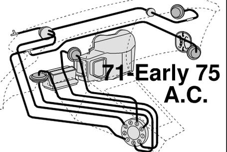
71-Early 75 A.C. Vacuum Hose Kit includes 9 color coded vacuum hoses, 2 T-pipe fitting, 18 clamps & a Full Color Schematic Diagram with Instructions. This kit is not used with a Hot Water Shut Off Valve. 9222106 28.95
