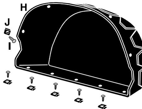
**H** 63-67 Assembled Glove Box Liner with Mounting Clips
