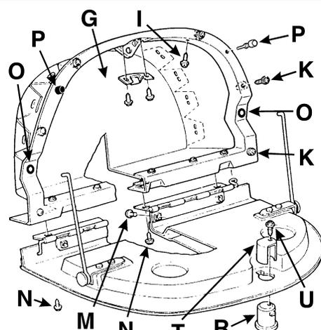
Glove Box Frame To Dash Mtg Hardware
